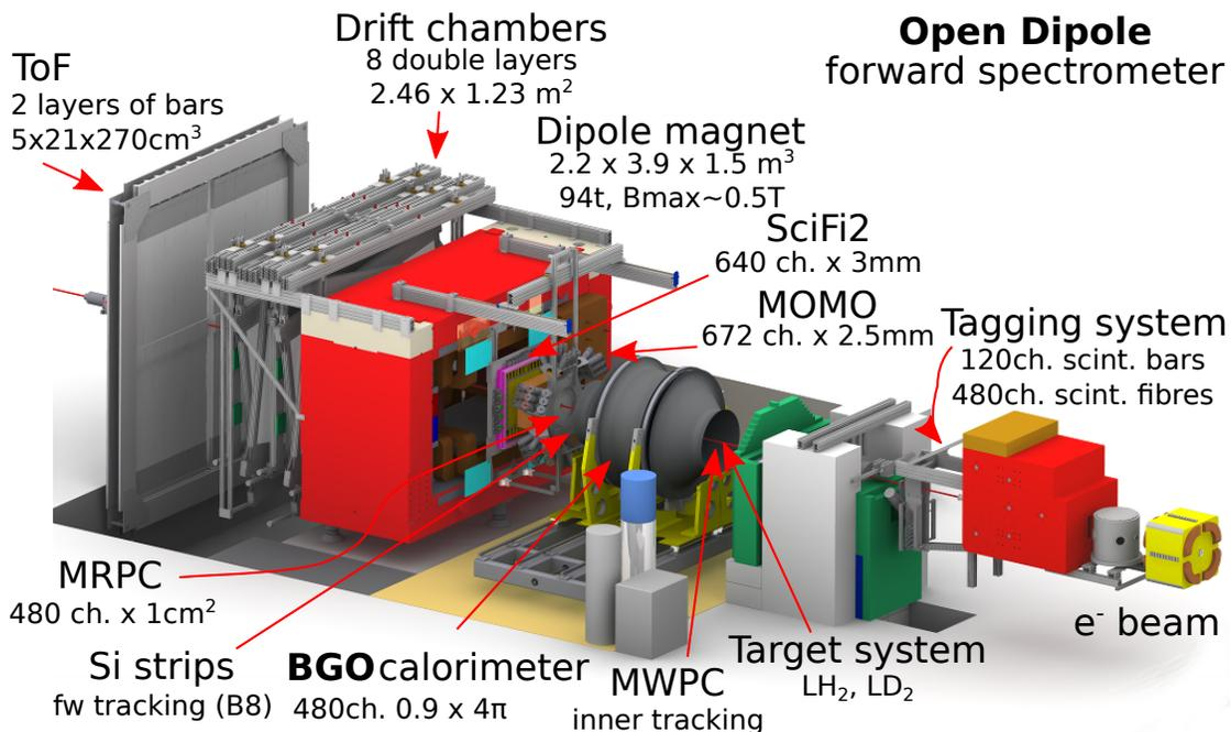
Figure 5 The BGO-OD experimental setup
