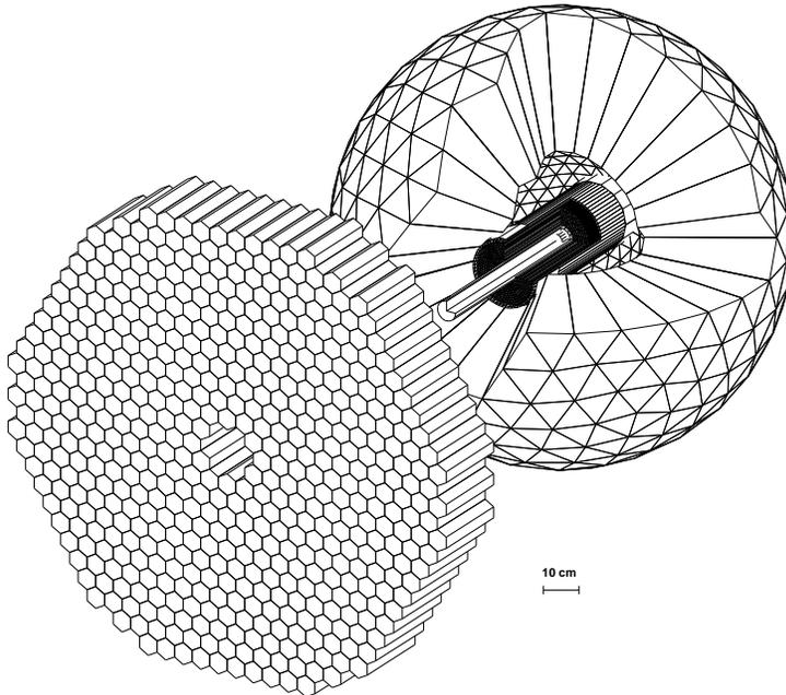
Figure 7: The experimental apparatus proposed for our measurements at MAMI. To show the position of the cylindrical wire chamber and the target inside the Crystal Ball some of the Crystal Ball crystals have been omitted.
