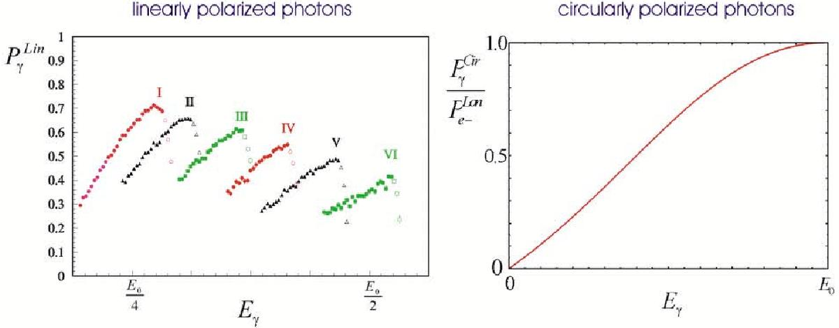
Figure 9: Energy distribution of linearly polarized photon beam at several goniometer settings.
