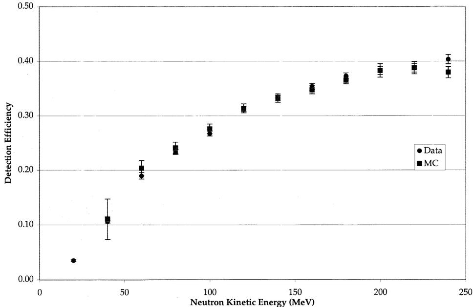
Figure 8: The neutron detection efficiency obtained with the Crystal Ball using the reaction  $\pi^- p \rightarrow \pi^0 n$  measured for four  $\pi^-$  beam momenta [St01].
