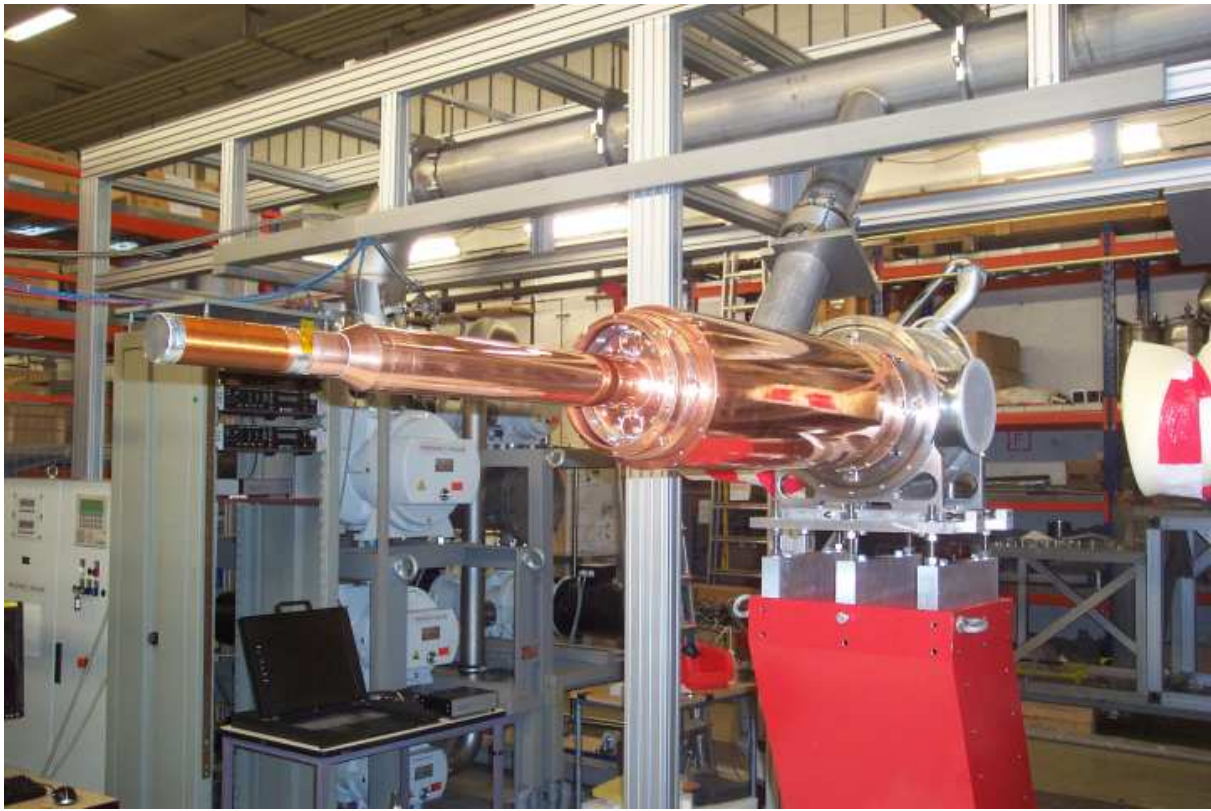
Figure 16: The new dilution refrigerator for the Crystal Ball Frozen Spin Target.
