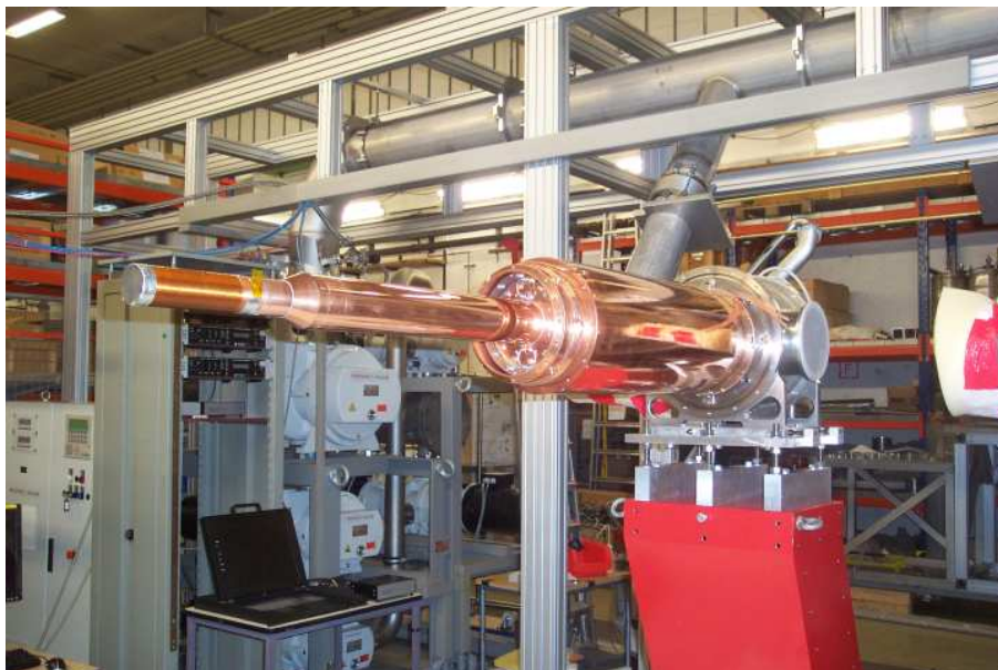
Figure 17: The new dilution refrigerator for the Crystal Ball Frozen Spin Target.
